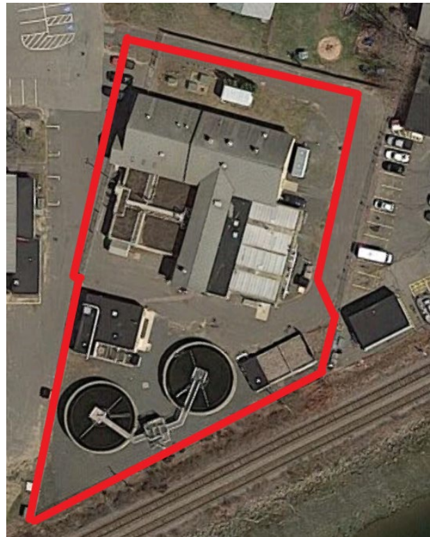
Figure 3: Flood Barrier Alignment at WWTP
