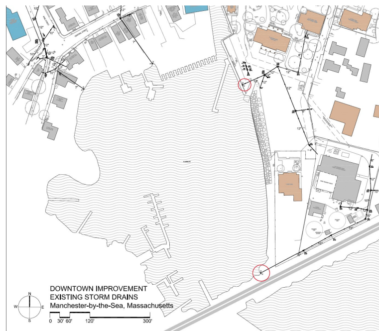
Figure 5: Locations of Stormwater Outfalls near WWTP and Town Hall
