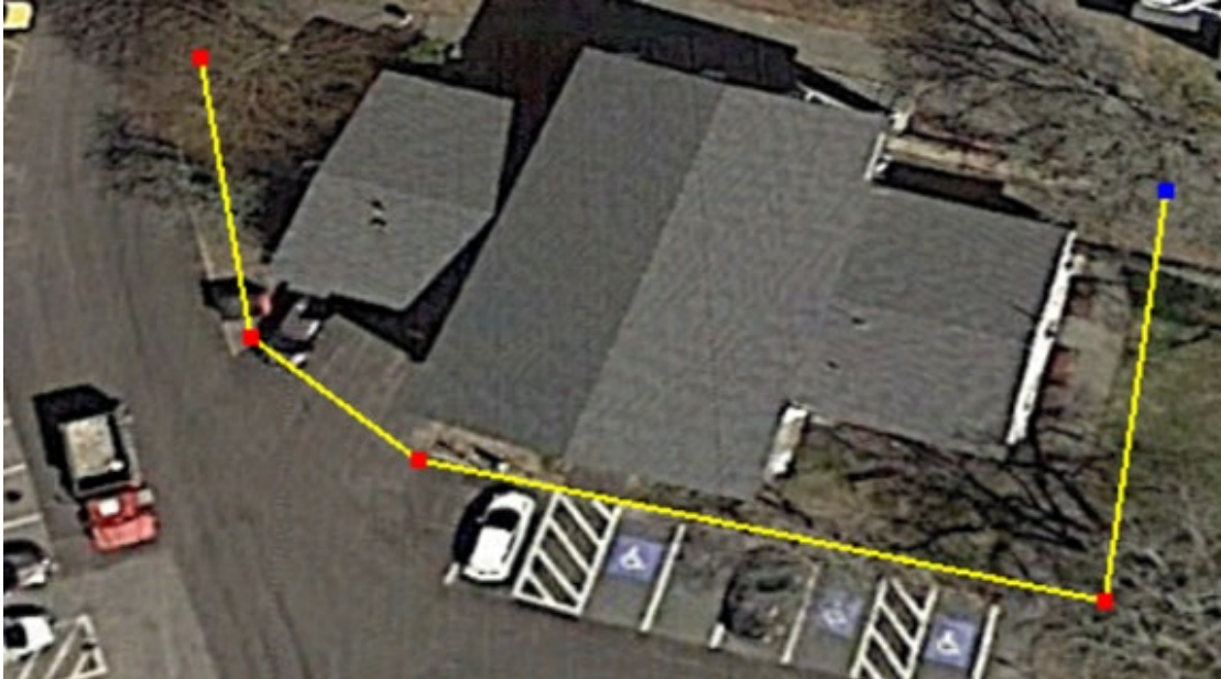
Figure 7: Flood Barrier Alignment at Town Hall/Police Station
