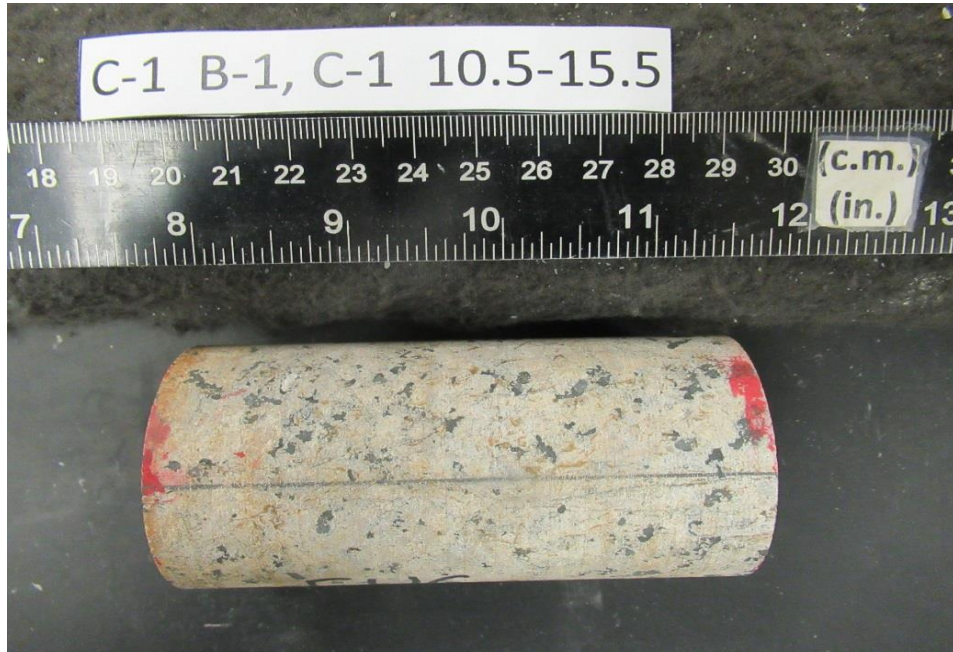
After cutting and grinding
